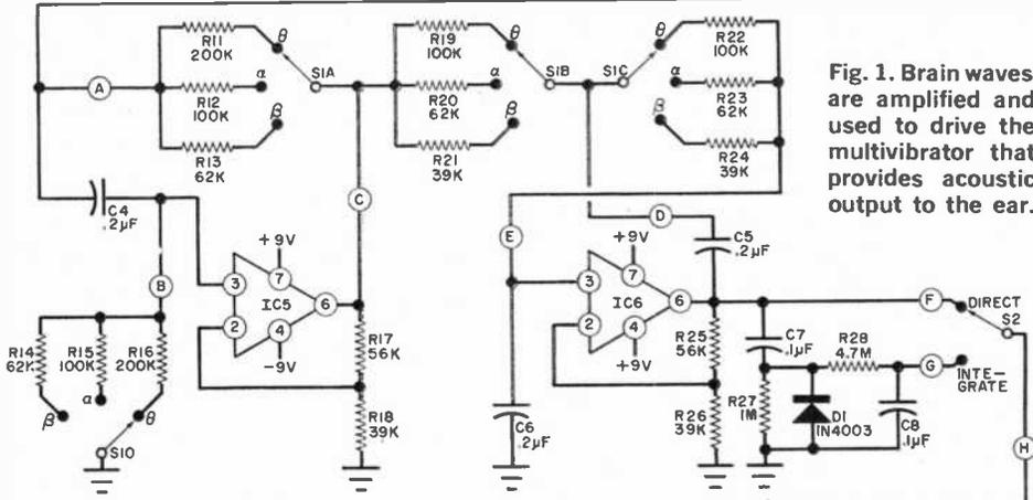
Fig. 1. Brain waves are amplified and used to drive the multivibrator that provides acoustic output to the ear.
